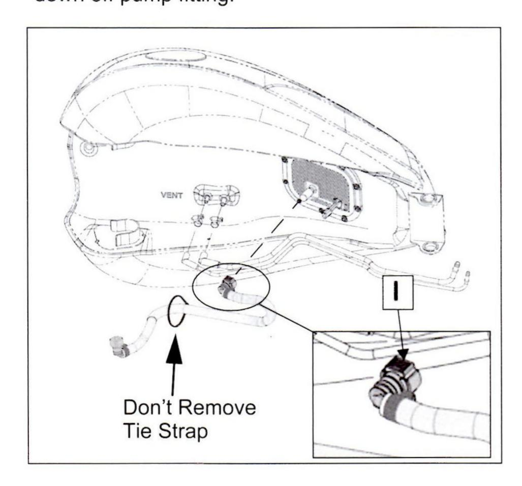
Install fuel tank fitting plug tool (see Special Tools for application details) onto fuel pump fitting to protect the fitting and prevent fuel for seeping out of tank.
